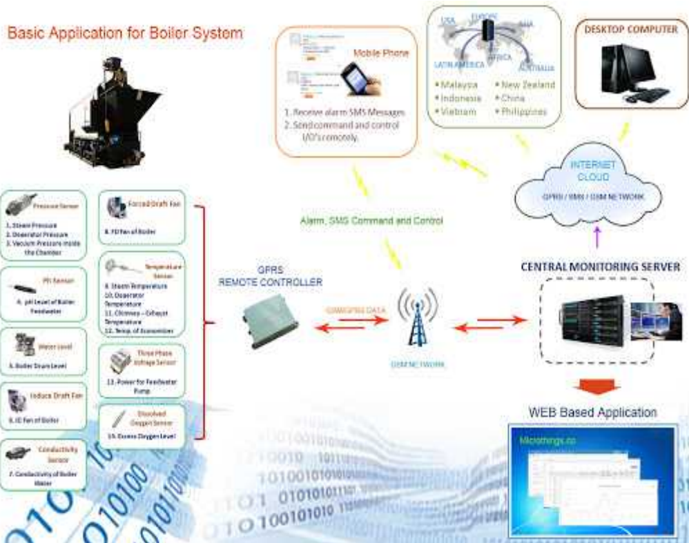
Example of GSM/GPRS Remote Controller
